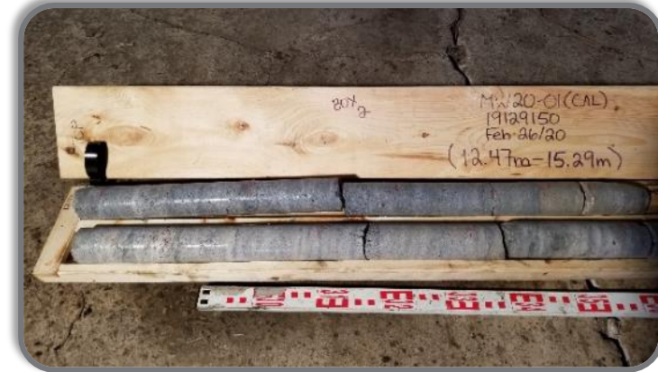
Rock core sampled during exploratory drilling
