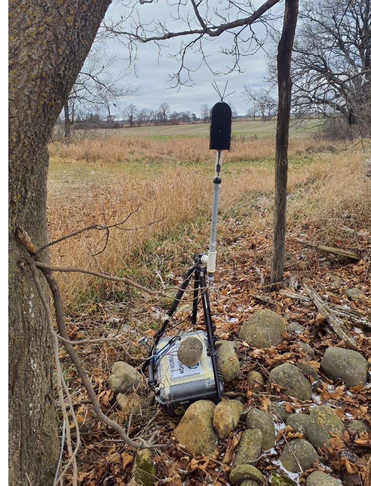
Baseline noise monitoring equipment deployed at the Project Location
